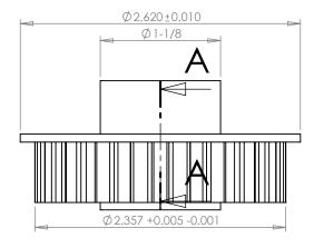
**NOTE: CORED PULLEYS** HAVE 1/16" THICK RIBS, REINFORCEMENT
